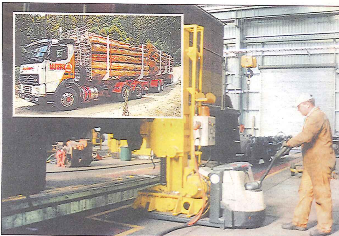
MAIN PHOTO — Adam Willis lifts a 2112 loco with a stationary lifting jack at Tasrail's motive power centre. INSET — Best practice in logistics has been executed by utilising Tasrail's long distance efficiencies of train haulage with Lloyds North's high productivity trucks featuring road-friendly suspensions.
