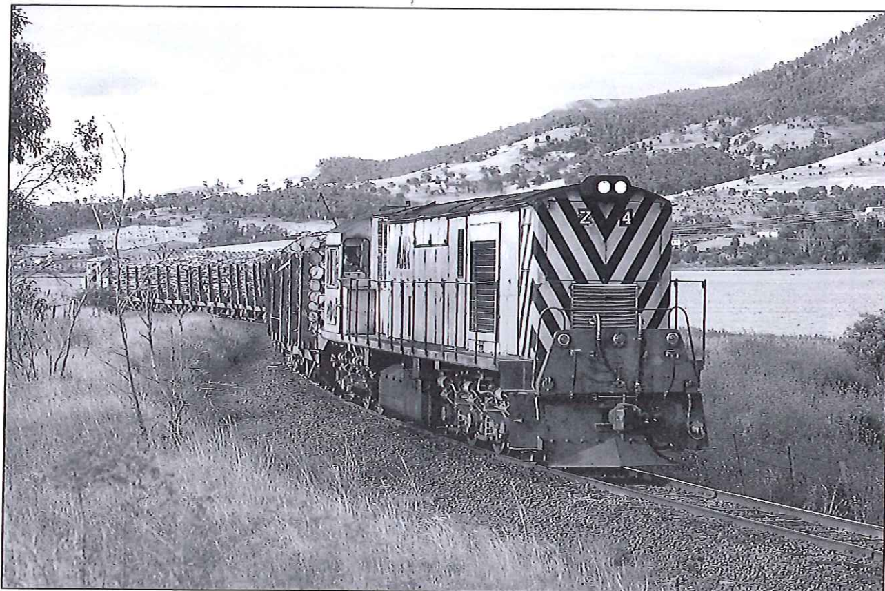
Z 4 heads a down train between Bridgewater and Boyer, running beside the Derwent River with a load of logs for the Australian Newsprint Mills. The four members of the Z class were built by English Electric in 1972 and whilst fitted with dual cab controls, it was unusual to see them running long hood leading. 17.4.85.
